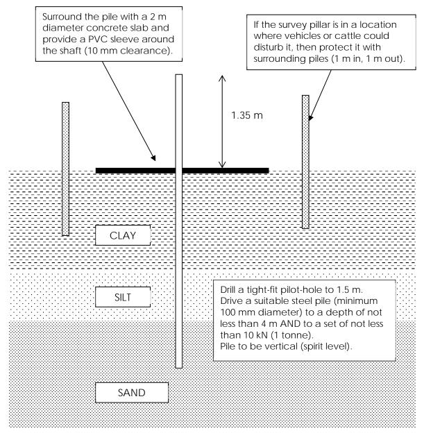
Figure D-1: Recommended Survey Pillar Construction for River Murray according to Geotechnical Conditions
