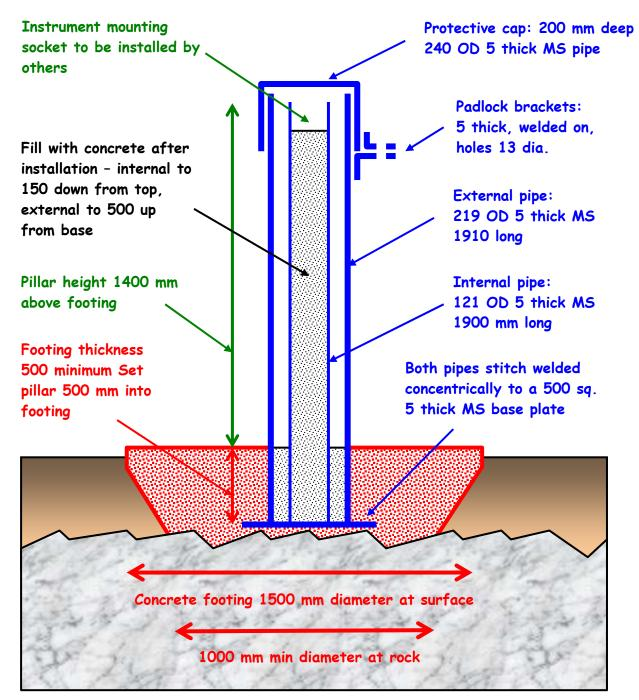
Figure 5-1: Standard Design for Shallow Rock Foundation
