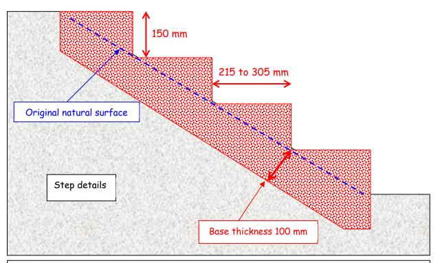
The "slope" of all flights of steps to be between 1:1.4 and 1:2 (35° and 26°) \*. All risers to be 150 mm high. Goings to be between 215 mm min and 305 mm max – but constant on each flight. Treads to be 800 mm wide and horizontal. The number of risers in any flight of steps should not exceed 18. Concrete to be N20 (normal grade 20 MPa) unreinforced\*.
