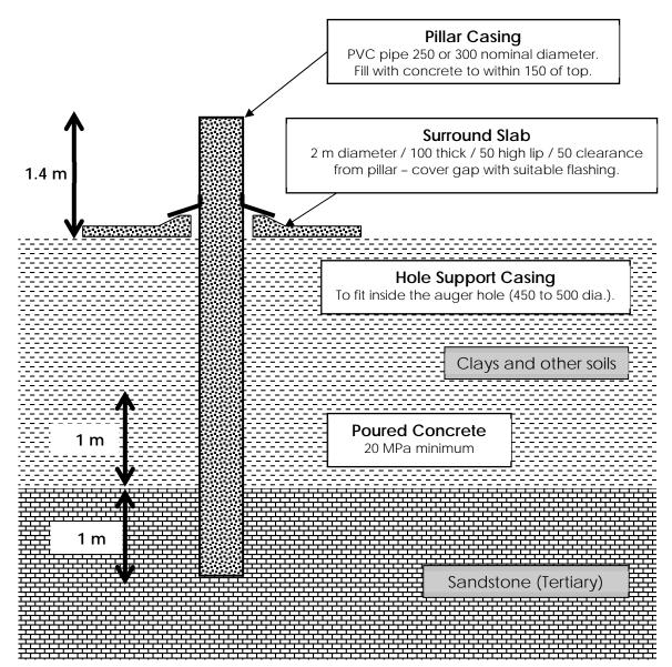
Figure E-1: Design example for Survey Pillars/ Permanent Benchmarks in Hope Valley Dam
