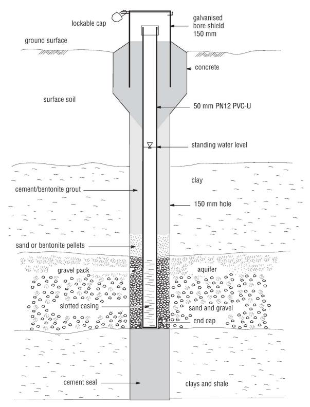
Figure 3: Minimum construction requirements of monitoring well (NUDLC, 2012)
