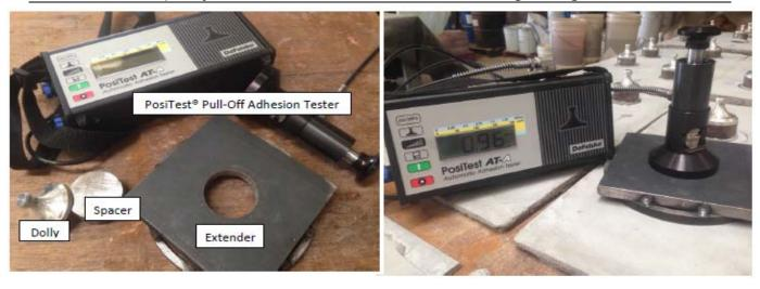
Figure 2 - Pull test apparatus and set-up.
